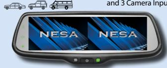
The 7" widescreen can display a rear camera and 2 side/blind-spot cameras. Triggered by either reverse gear or indicators, the screen will display the camera automatically or can display a specific camera manually with the soft touch controls on the left of the screen. Manually switch between rear, left or right, or both left and right together. The screen is invisible when not in use, so looks like a standard mirror. Connect any cameras with RCA plugs.
