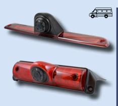
Available in vehicle specific (Sprinter, Transit, Ducato) and non-specific universal mounting. The Mercedes and Ford models have a high resolution CCD sensor. the Fiat and universal models use a CMD sensor. All models are encased in a ball'n'socket style housing for versatile view angle adjustment. Simple installation with no additional drilling is
