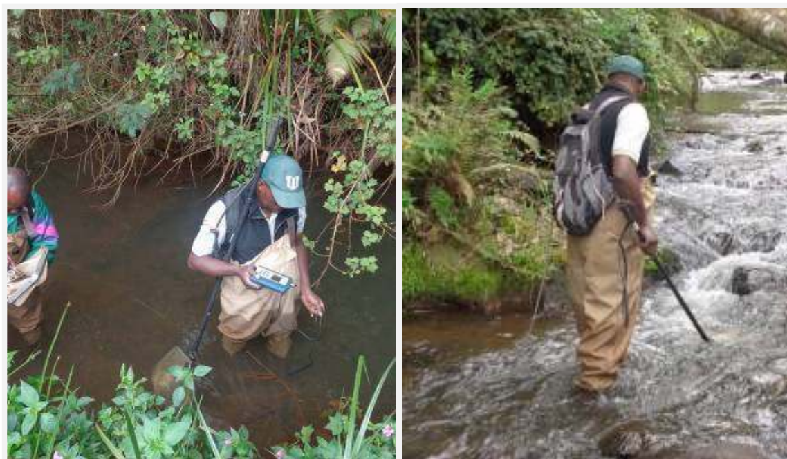
Figure 1-5: Measuring water quality parameters in a pool and sampling of fish using Electrofisher in a riffle
