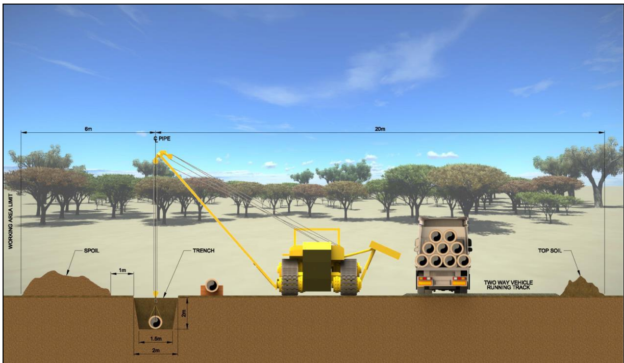
Figure 2-10: Typical Right of Way along the pipeline route during construction (photo courtesy)
