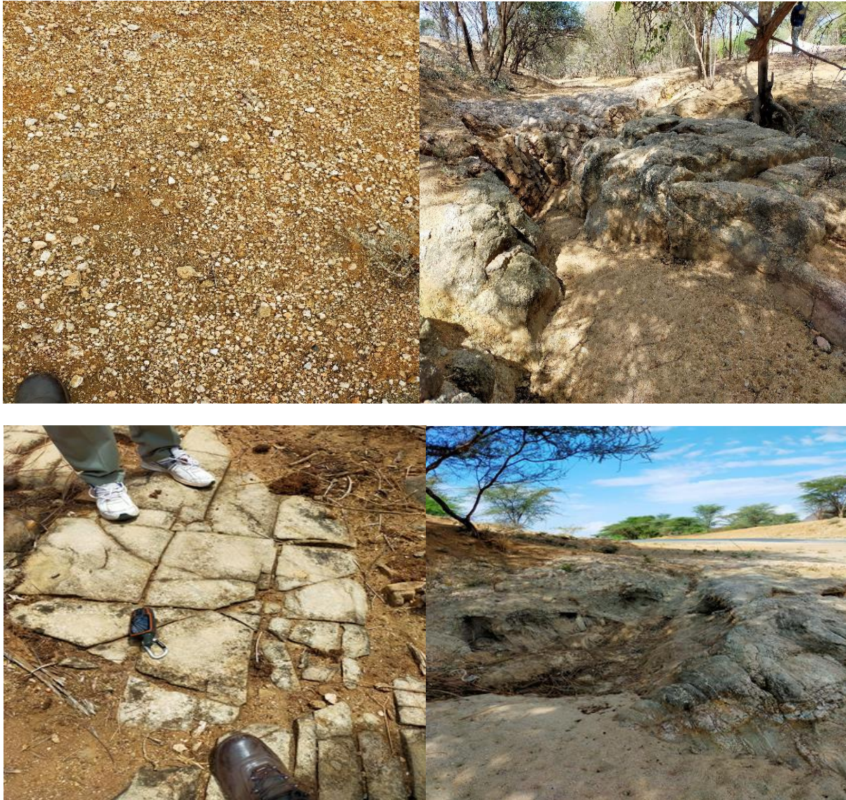
Plate 5-7: Rock exposures within Lokichar/Loperot Mesozoic basin along the water supply pipeline route on Kapenguria - Lodwar road. Top: Left to right: Quartz rubbles/pebbles and pegmatite within biotite gneiss, Bottom: Leucocratic biotite gneiss grading to more melanocratic biotite gneiss exposures
