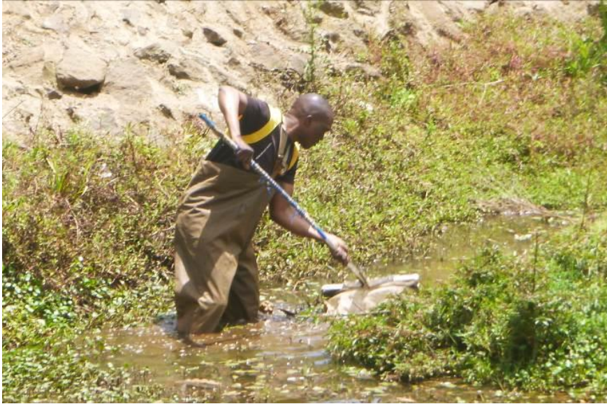
Figure 1-1 Sampling of aquatic macro-benthic invertebrate using kick-sampling method with pond net
