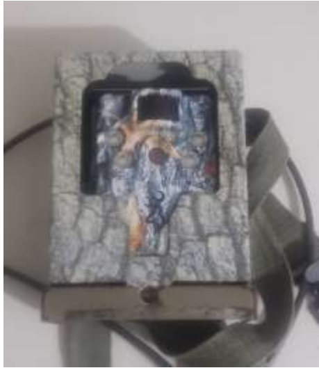
Figure 5-35: Browning Trail Camera in a security box
