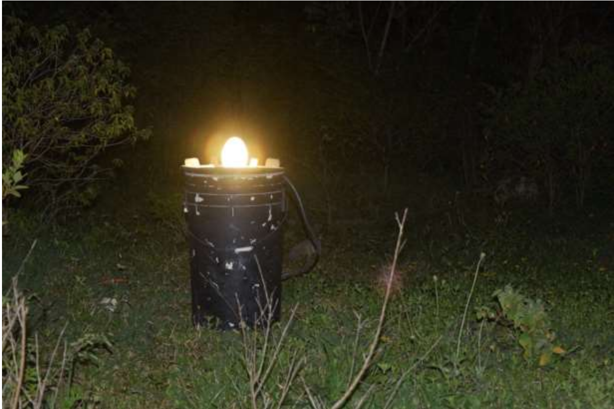
Figure 5-40; Modified Robinson's light trap, fitted with a 175-watt Mercury Vapour collecting light bulb and a funnel with baffles
