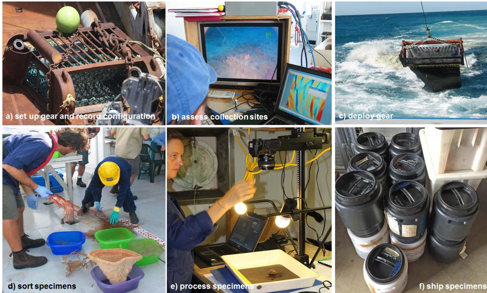
Figure 8.1 Images from key steps involved in the use of benthic sleds and bottom trawls for marine monitoring: a) a modified WHOI sled with attached pipe dredges, b) seafloor imagery from towed video and bathymetric grids, c) lowering the AIMS benthic sled, d) sorting animals on the back deck, e) photographing specimens in ship laboratory, f) securely sealed containers to ship animals to museums
