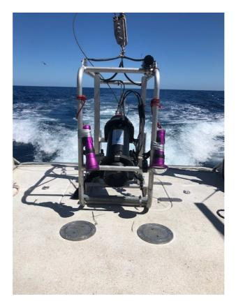
Figure 3-1. NSW DPIE Towed Video fish setup showing centred forward-looking video camera with live fish-tosurface fibre optic feed and lights, rear deck of RV Bombora (the digital stills camera sits toward the back of the tow-frame and not visible here).
