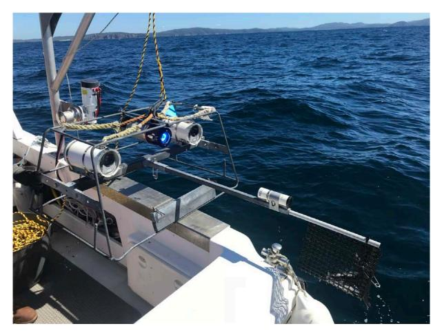
Figure 4-4. An example of a baited remote underwater stereo-video unit, including blue light, used in this study.
