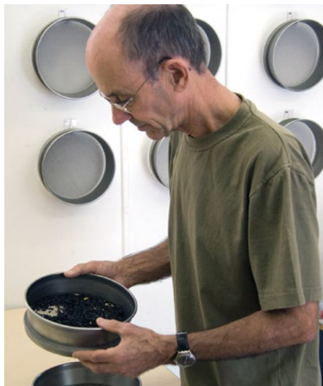
Figure 6.9 Seeds can be separated from fruits, chaff, and other non-seed material using sieves. (Photo: A Crawford)
