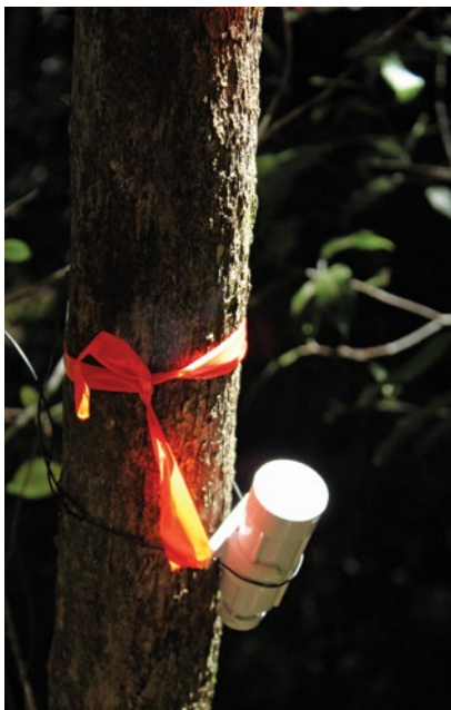
Figure 8.18 Climate logger at Wollemi Pine site. (Photo: C Offord)
