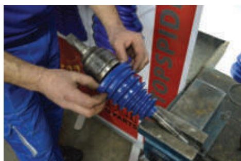
10. PUT THE CV BOOT BACK TO THE ORIGINAL CONDITION / Manžetnu vratiti u prvobitno stanje
