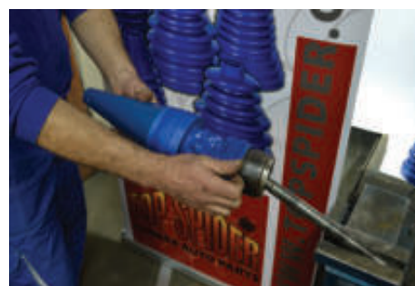
8. PUT THE SLIDER COMPLETE WITH THE CV BOOT ON IT ON THE JOINT / Levak sa manžetnom nabaciti na HKZ
