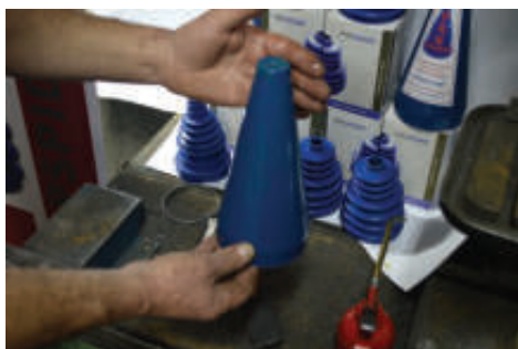
4. SPREAD ON OIL ON THE SLIDER / Namazati levak uljem ili tečnim silikonom
