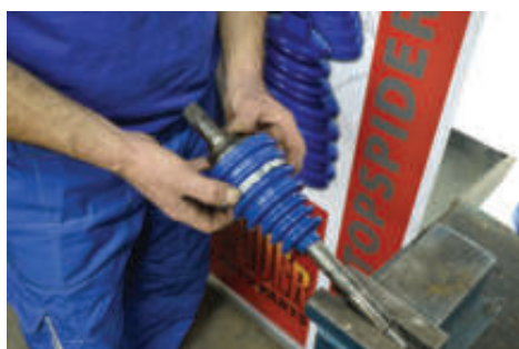
11. USE THE GREASE AND PUT THE CLAMPS ON / Staviti grafitnu mast i montirati šelne
