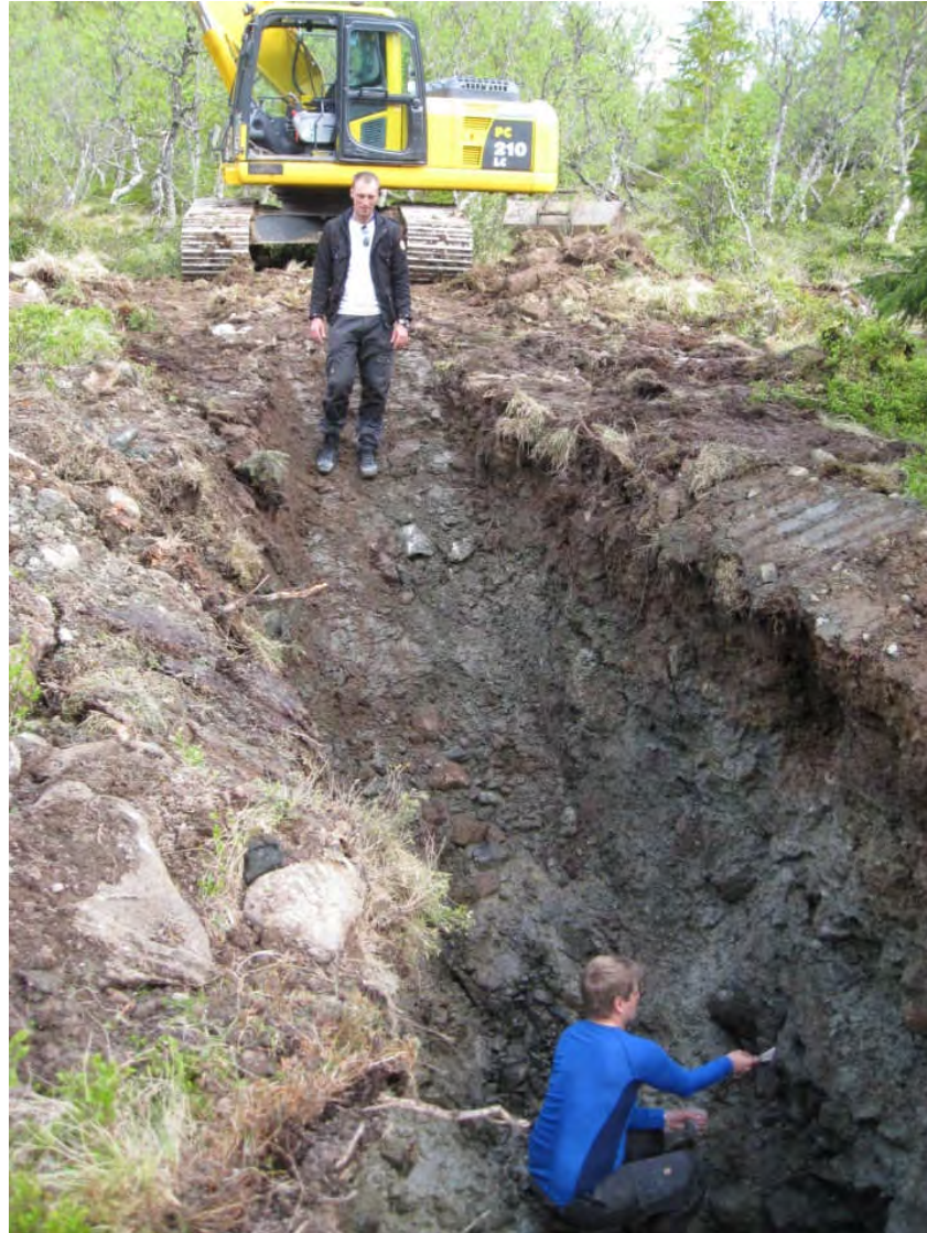
Figure 6.14 Excavation at Sortland. We observed fractured basement with minor signs of weathering.
