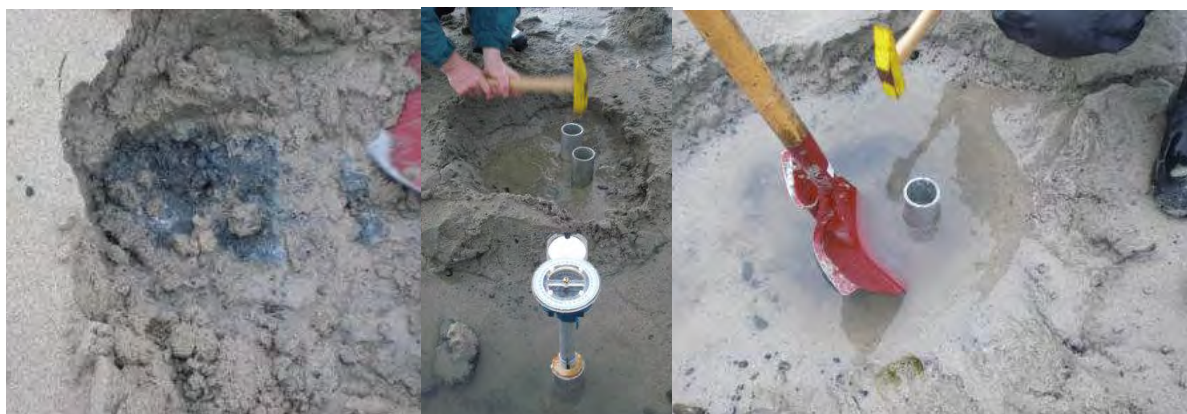
Figure 2.8 Oriented sampling of unconsolidated weathered bedrock at Ramså, Andøya.
