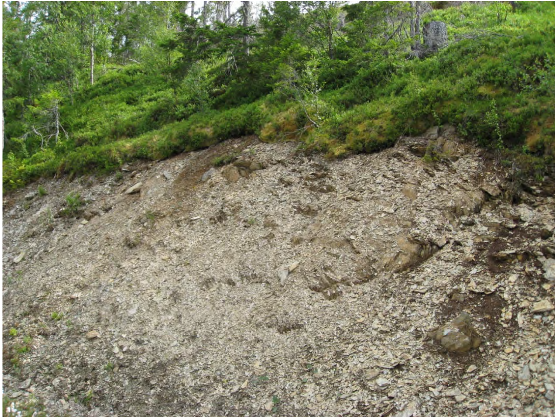
Figure 5.35 Fractured and fragmented mica schist along a road-cut at Dørgåsen in Mosvik (UTM 32, WGS84 593800-7078550). The clay content appears to be low even though the rock seems to be totally disintegrated. This type of weathering is typical for the soil that is identified as weathered material (forvitningsmateriale) on the Quaternary map (Reite 1997, Sveian & Solli 1997, Sveian 1985, Sveian et al. in press).
