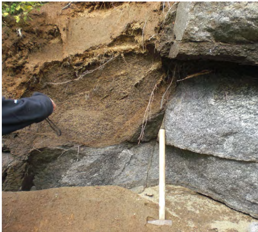
Figure 6.38 Example of a very sharp transition between weathered and fresh bedrock at a road-cut on Hamarøya.
