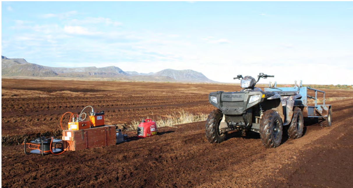
Figure 2.1 Acquisition of electric resistivity data south of Ramsåa at Andøya (Andøyatorv peat extraction plant).
