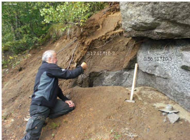
Figure 2.5 Magnetic measurements of weathered and un-weathered bedrock on Hamarøya. The remaining magnetisation of the altered rocks is reduced to a third compared to the parent material.
