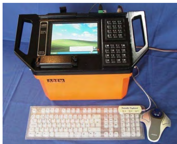
Figure 2.4 The seismic recording system ABEM TERRALOC MK6.
