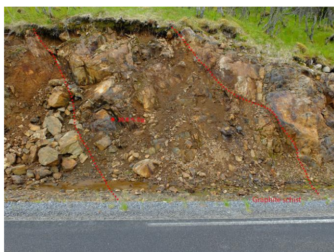
Figure 19. Picture from one of the road cuts in Romsetfjorden, an example of the outcropping graphite schist.
