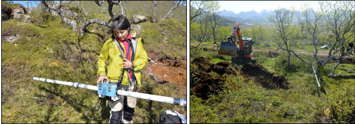
Figure 4. Pictures showing the EM31 electromagnetic recorder and trenching where conductors are located below soil cover (Photo: left Bladet Vesterålen, right NGU).
