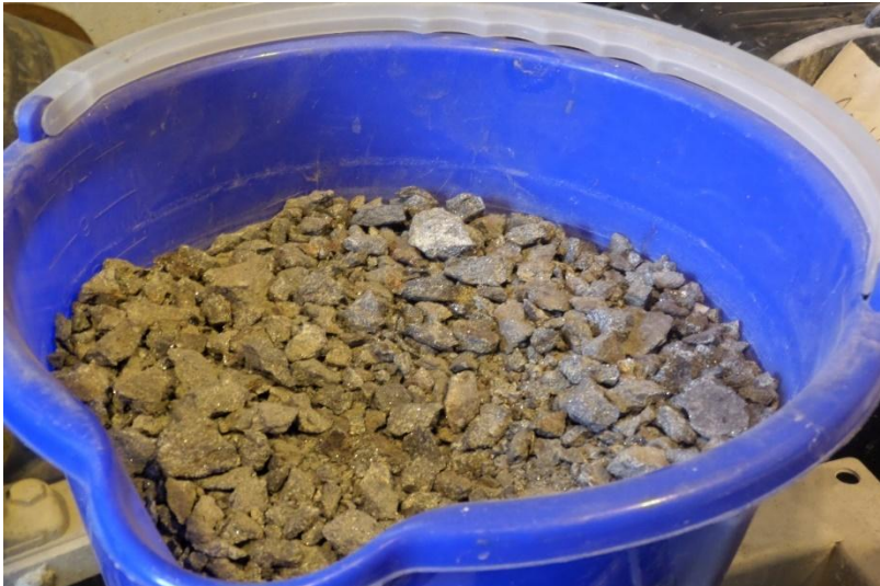
Figure 23. Crushed graphite schist before beneficiation trials.
