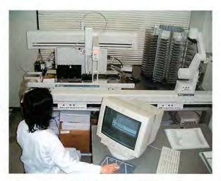
Figure 2. Biomek 2000 Laboratory Automation System.
