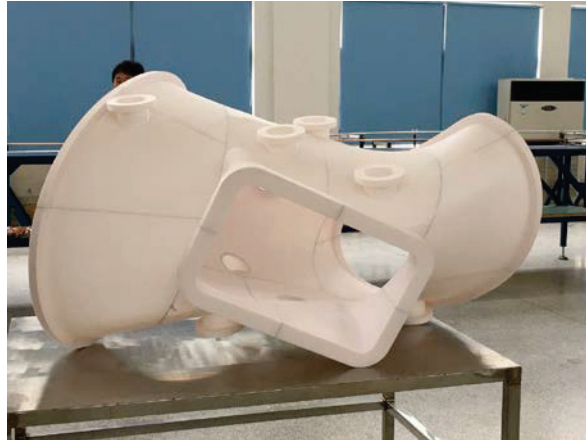
Fig. 11 Real scale vacuum vessel model made by 3D printer
