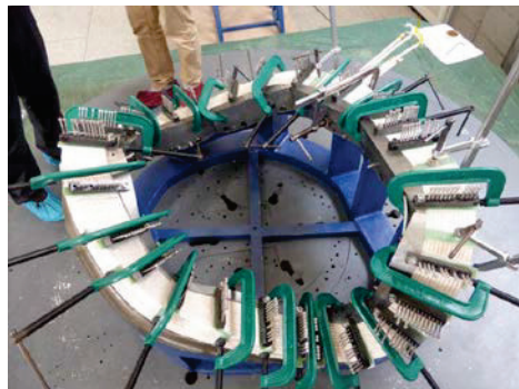
Fig. 6 Picture of mockup coil just after winding process of copper conductor, which was wrapped with fiber glass and Kapton tape, was completed.
