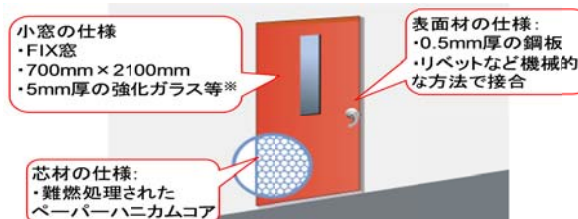
Figure 2 Fire safety facility used in semi-vertical sections (blocks fire for ten minutes)
