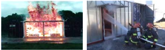
Figure 4 Actual measurement of fire extinguishing effect on main structural parts
