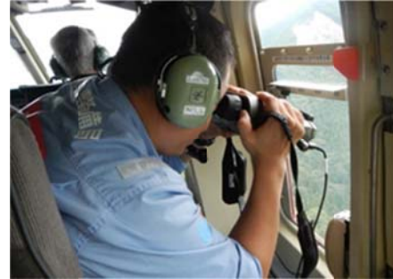
Photo 1. Training of laser distance measurement from the helicopter at the site of an actual landslide dam
