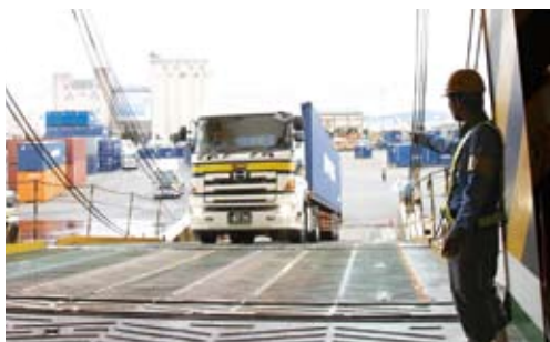
A container on a container chassis being loaded on board the roll-on, roll-off (RORO) cargo ship, Himawari .
