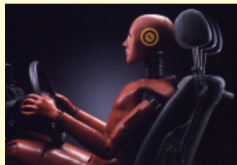
An Active Head Restraint for both the driver and front passenger seats is designed to help reduce whiplash neck injuries in traffic accidents.
