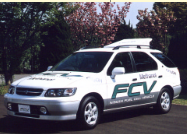
Nissan developed and began driving tests of a fuel cell vehicle equipped with a methanol reformer to generate hydrogen from methanol as the fuel.
