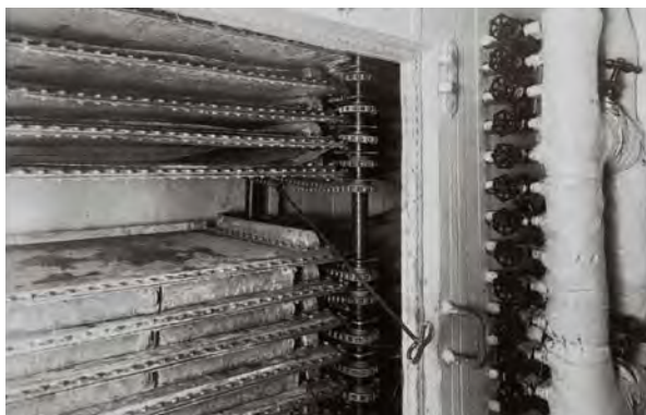
Iwamoto on-board rapid freezer Each tank could be raised or lowered individually
