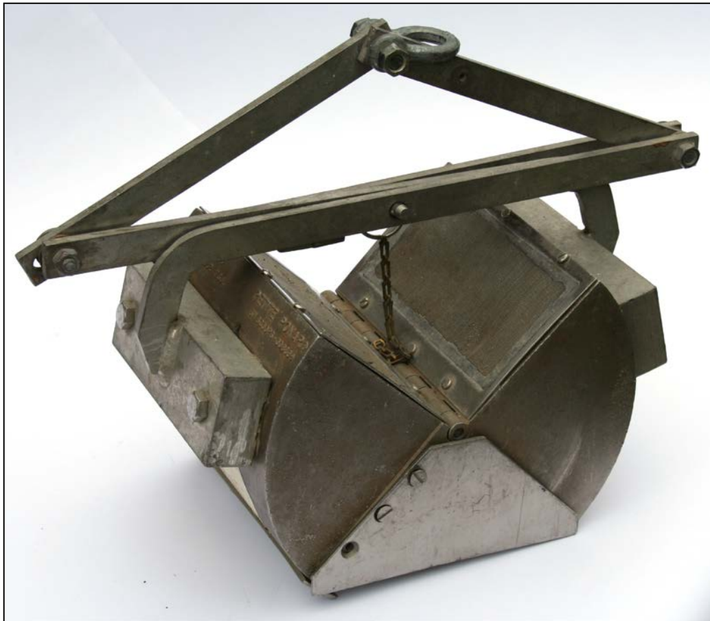
Figure 5. The petite ponar grab sampler. The sampler is lowered to the bottom of the waterbody, freefalling for the final meter to allow penetration of the bottom sediment. Upon reaching the bottom, the closing mechanism is activated. As the sampler is retrieved, it encloses a portion of the substrate.
