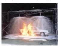
Foam Extinguishing Test
