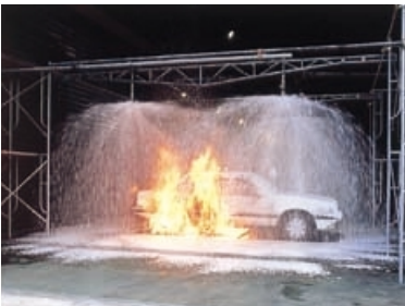
Foam Extinguishing Test
