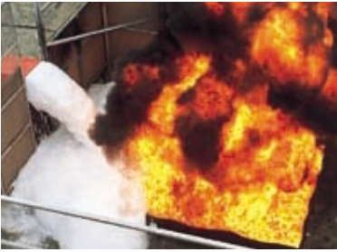
High-Expansion Foam Extinguishing System
