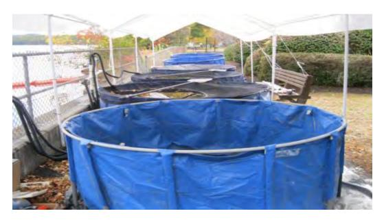
Figure 4-14 Fish holding tanks continuously supplied with ambient river water by two redundant pump systems connected to different electrical circuits, and were numbered to clarify test dates.
