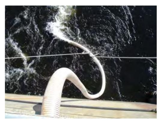
Figure 4-10 The induction apparatus connected to 4-inch diameter hoses which allowed the shad to pass to the desired release points.
