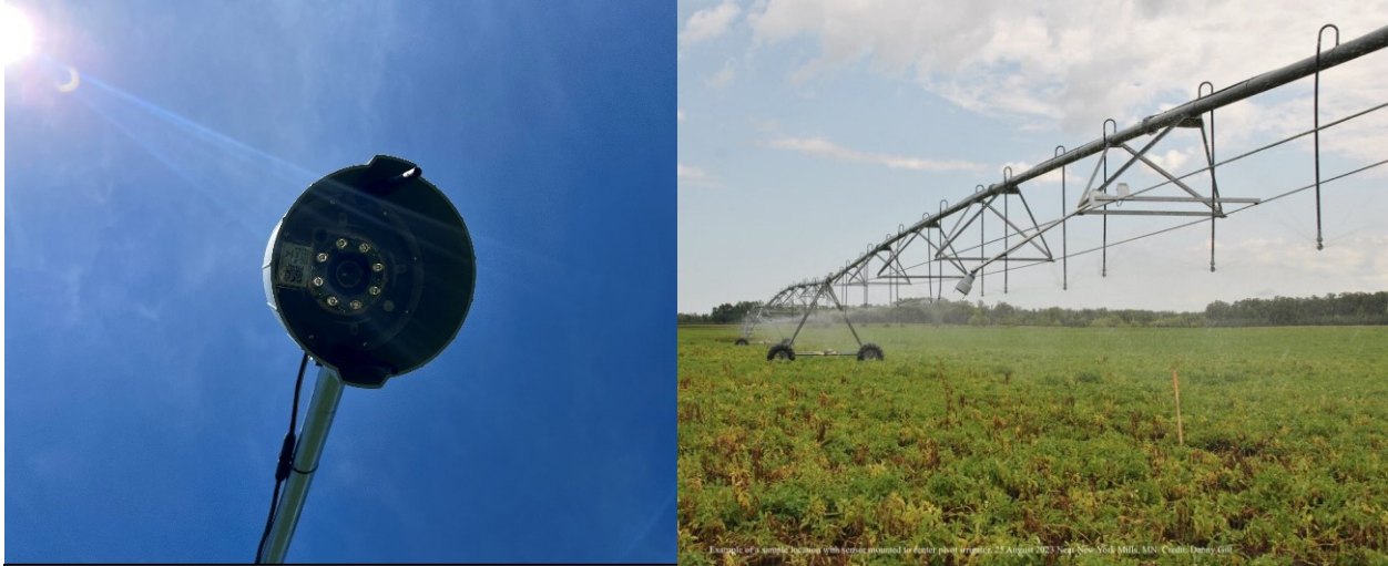
Figure 2. Left – View looking up at a camera attached to the irrigator used to visualize the crop throughout the growing season.
