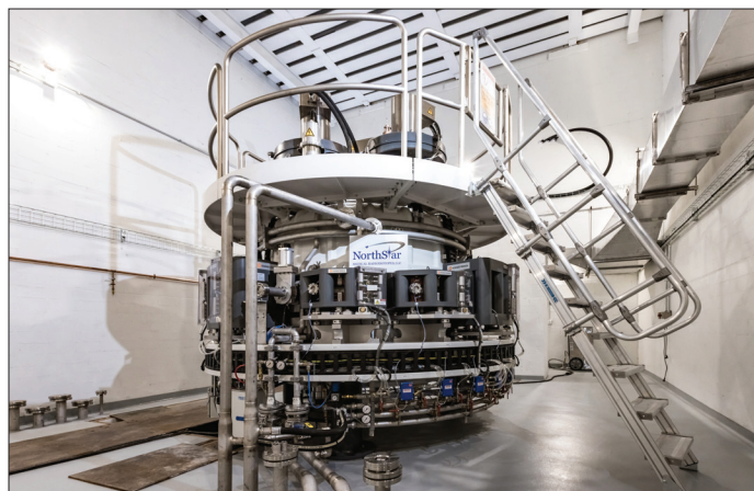
Figure 2. Ion Beam Applications (IBA) Rhodotron® TT300-HE electron accelerator, located in NorthStar's Ac-225 production facility, Beloit, WI.
