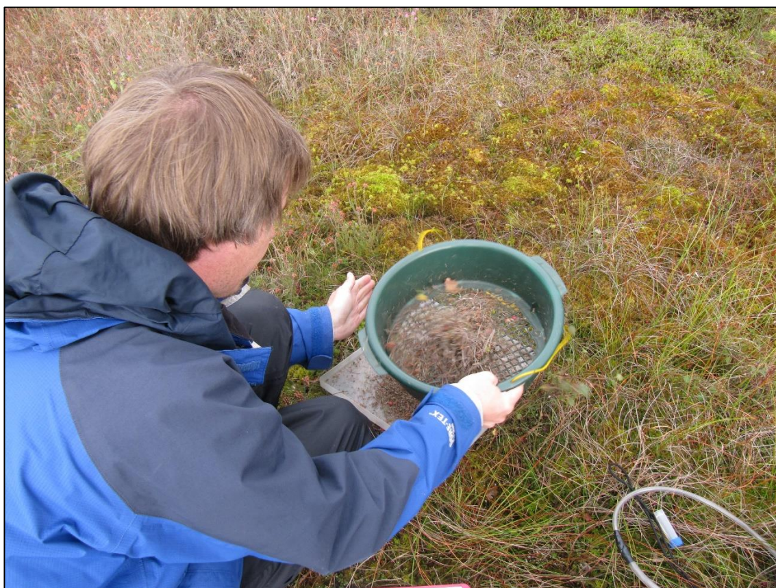
Figure 2. Sieving vacuumed sample over plastic tray to concentrate the sample.
