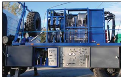
Truck mounted PTU and grease and hydraulic control module
