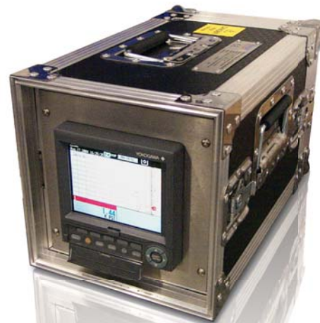
Electronic chart recorder part number L-6901004669
