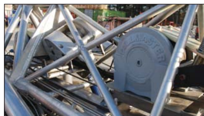
Utility winch and sheave lock winch
