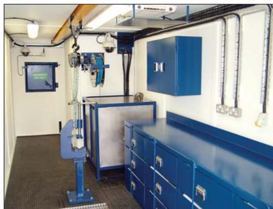
Workshop with test unit, Baker vice and chain hoist
