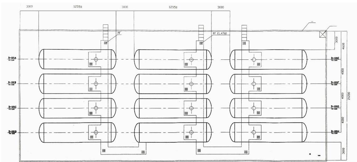
**Figure 2-21 Fuel storage tank layout**
