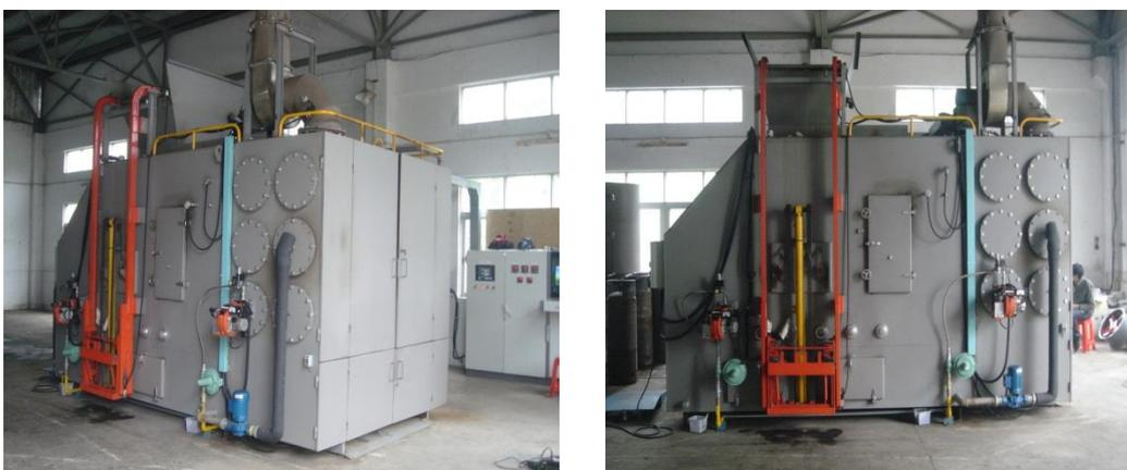
Figure 3- 17 Magnetization pyrolysis furnace
