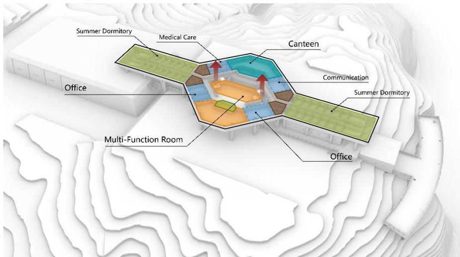
**Figure 2- 14 Functions zones of the first floor of the main building**
