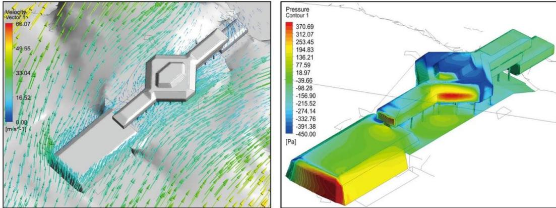
Figure 2- 19 Architectural appearance optimization with CFD modeling
