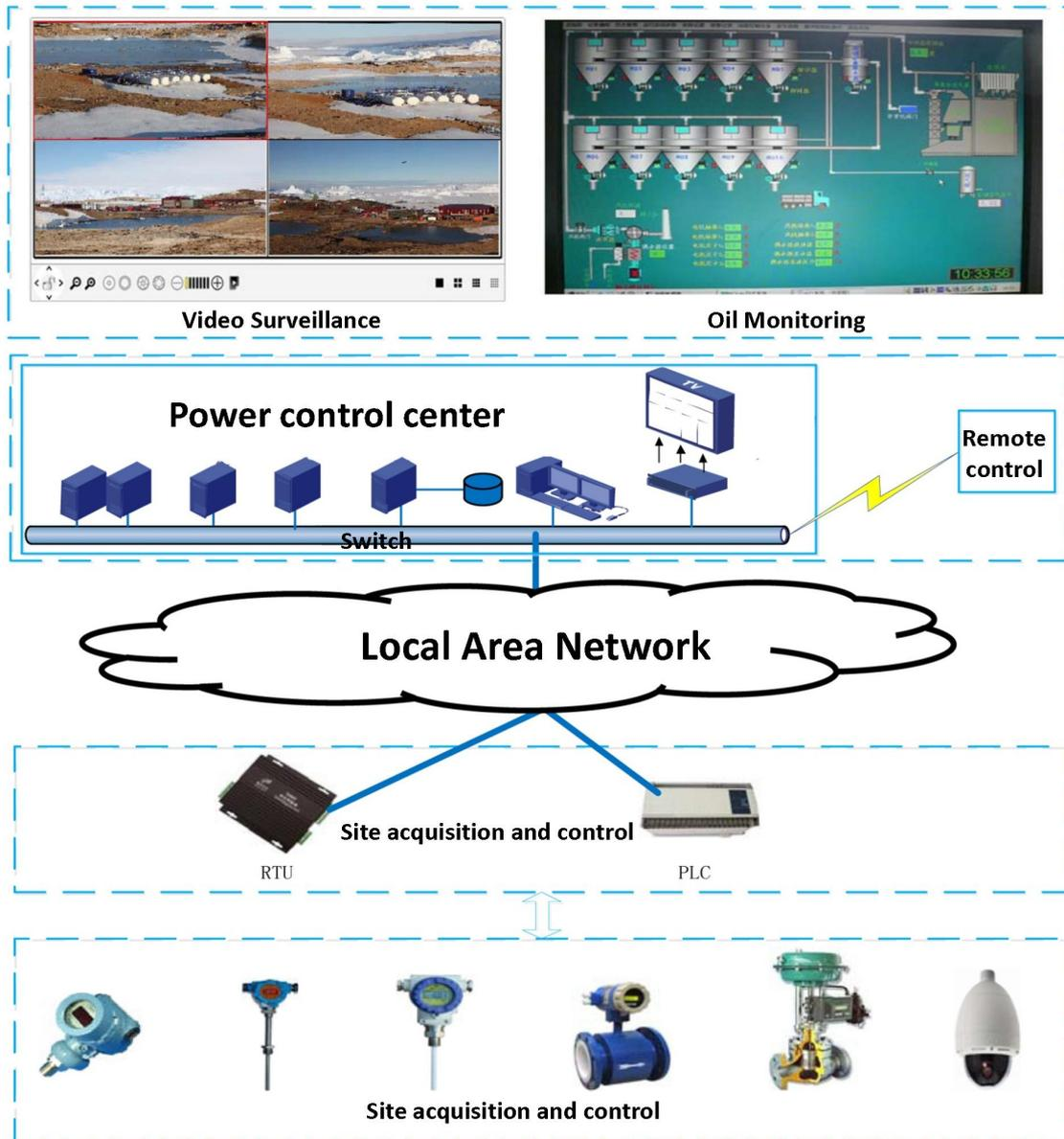
Figure 2- 20 Intelligent Monitoring System of the fuel storage system
