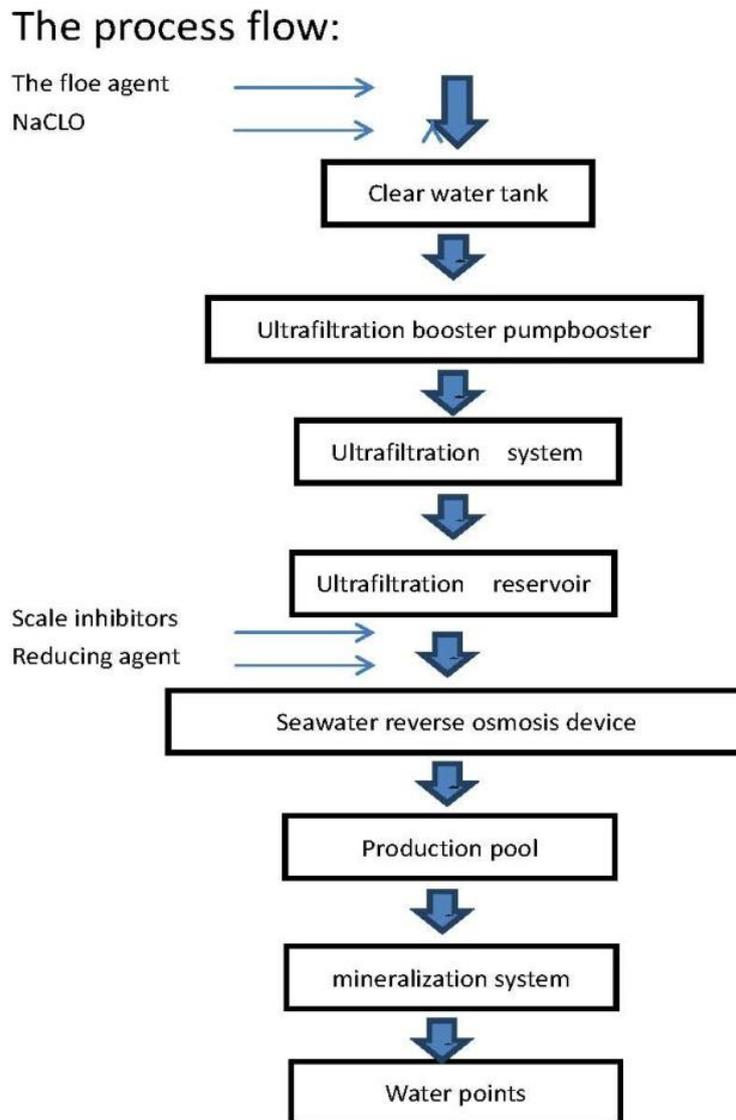
Figure 2- 27 Diagram of the SWRO system
