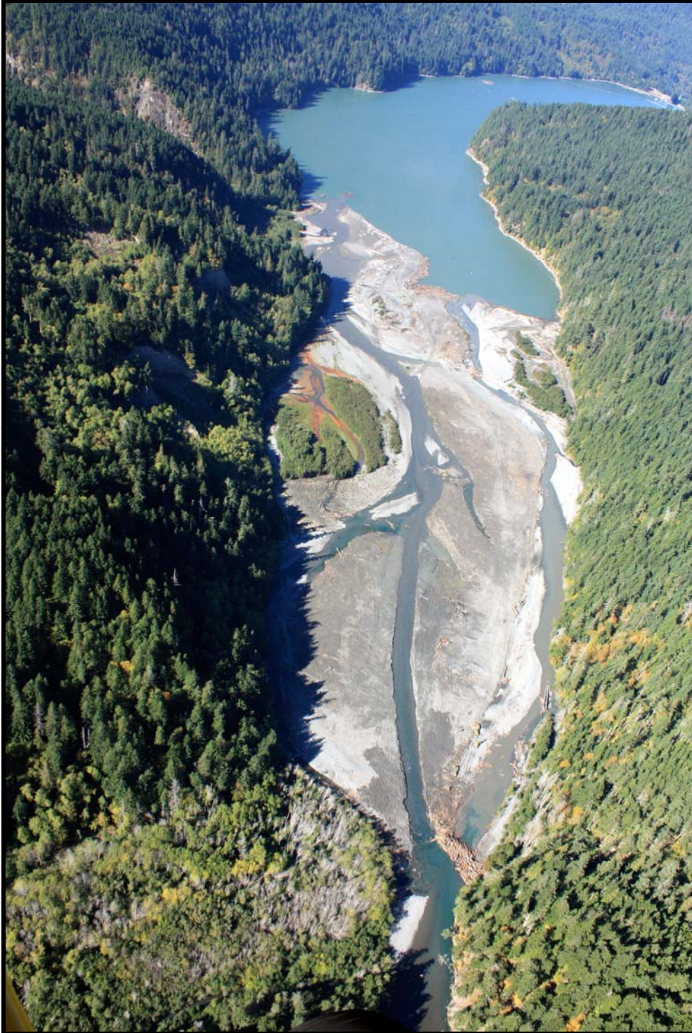
Figure 134. Aerial photograph of the sediment-built delta behind the Glines Canyon Dam on Lake Mills. Image taken just following completion of the first pre-removal construction tasks—carving a channel through the delta and the removal of the glade of alder trees covering it—at the dam site. September 2010. Photograph by Tom Roorda. Courtesy of Tom Roorda, NTI. [Roorda_IMG_5242.JPG]
