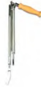
A sling psychrometer is relatively inexpensive but is not as accurate as a motor-driven model
