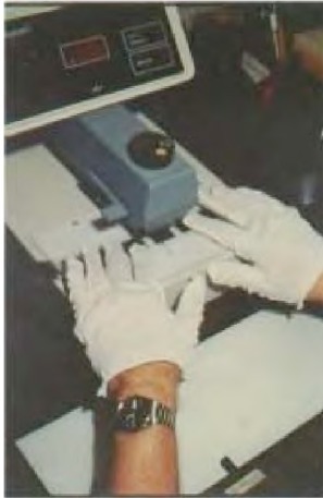
Quality control inspection of master microfilm will help ensure your copies are complete, fully readable, and chemically stable
