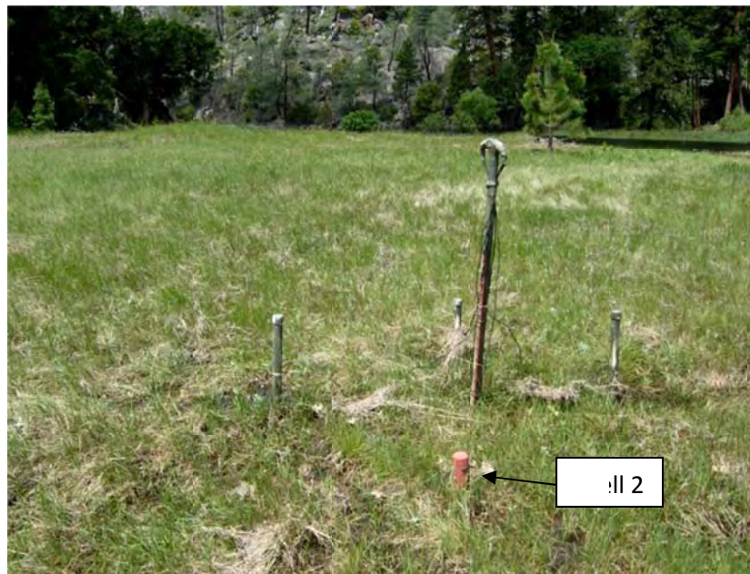
Figure 2-2. Soil moisture content measurement array at well 2. The three sensors surround the fence-post which served as means of elevating wiring junctions above the potential inundation level. Sensors were wired to a Campbell Scientific CR1000 datalogger located on a high point nearby (to left of this photo).
