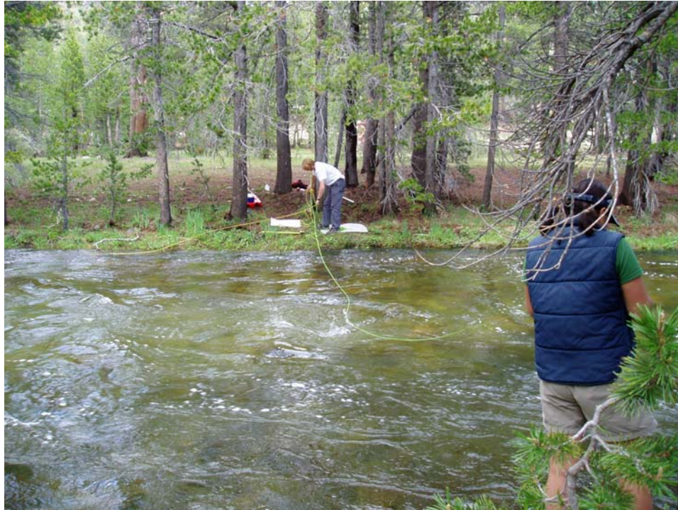
Figure 2-20. Bank full flow on Dana Fork of Tuolumne River near Bug Camp, 6/28/2006. Q=424 cfs.
