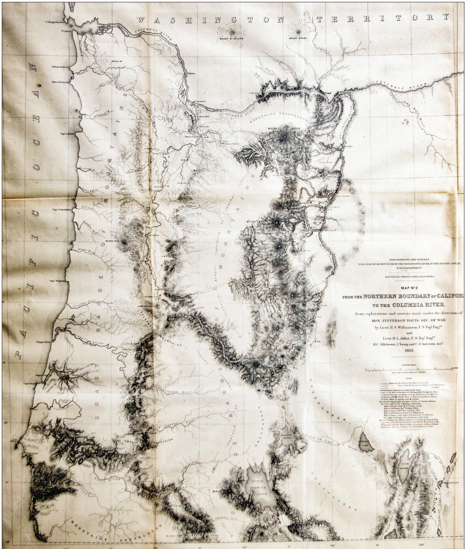
Map of the region from California to the Columbia River, drawn by the Williamson and Abbot survey crew (Abbot 1857). Note that some areas are mapped in great detail, while others are "unexplored;" for example, Crater Lake does not appear on their map. The area west of the Cascade peaks is labeled "Heavily timbered Ridges separated by immense ravines."
