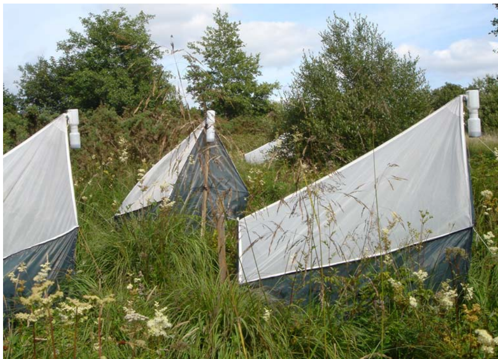
Figure 18: Large emergence traps. Each trap covers a ground-surface area of c.4sq.m. Attachment of the collection bottles is the same as for the small emergence traps. The large traps are required where ground vegetation grows higher than 50cm.
