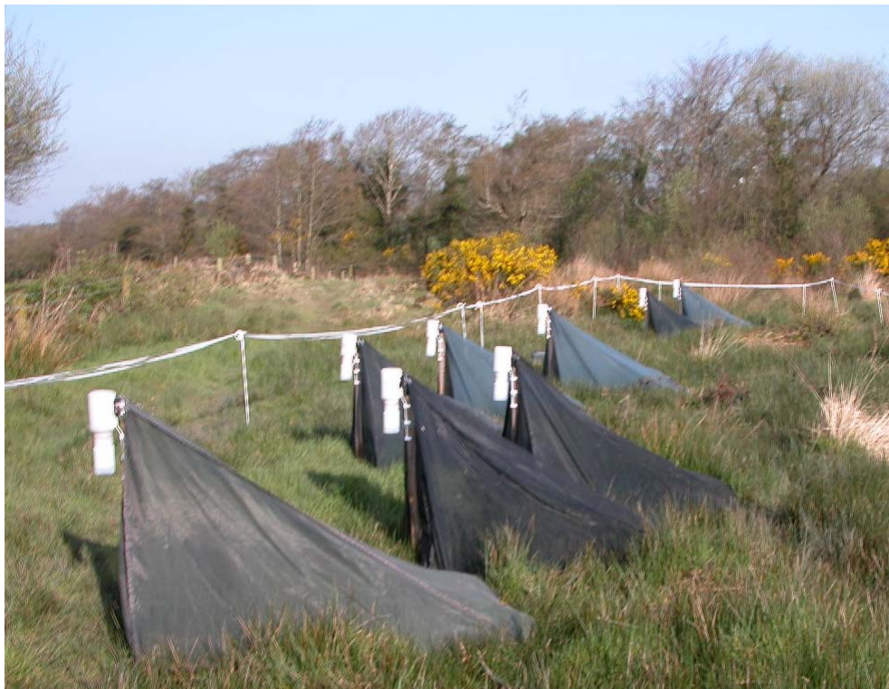
Figure 17: Small emergence traps. Each trap covers a ground-surface area of c.1sq.m. The small emergence traps can only be used efficiently where the ground vegetation is no more than 50cm high. Syrphids and other insects emerging within a trap are collected in alcohol, in the lower of the two bottles connected to the trap at its highest point. Connection is achieved by means of a tube running between the interior of the trap and the upper collection bottle. The tube is open at both ends, allowing insects to move from inside the trap into the collecting bottles. The lower collection bottle can be unscrewed from the upper bottle and removed, containing its sample of emerged insects.
