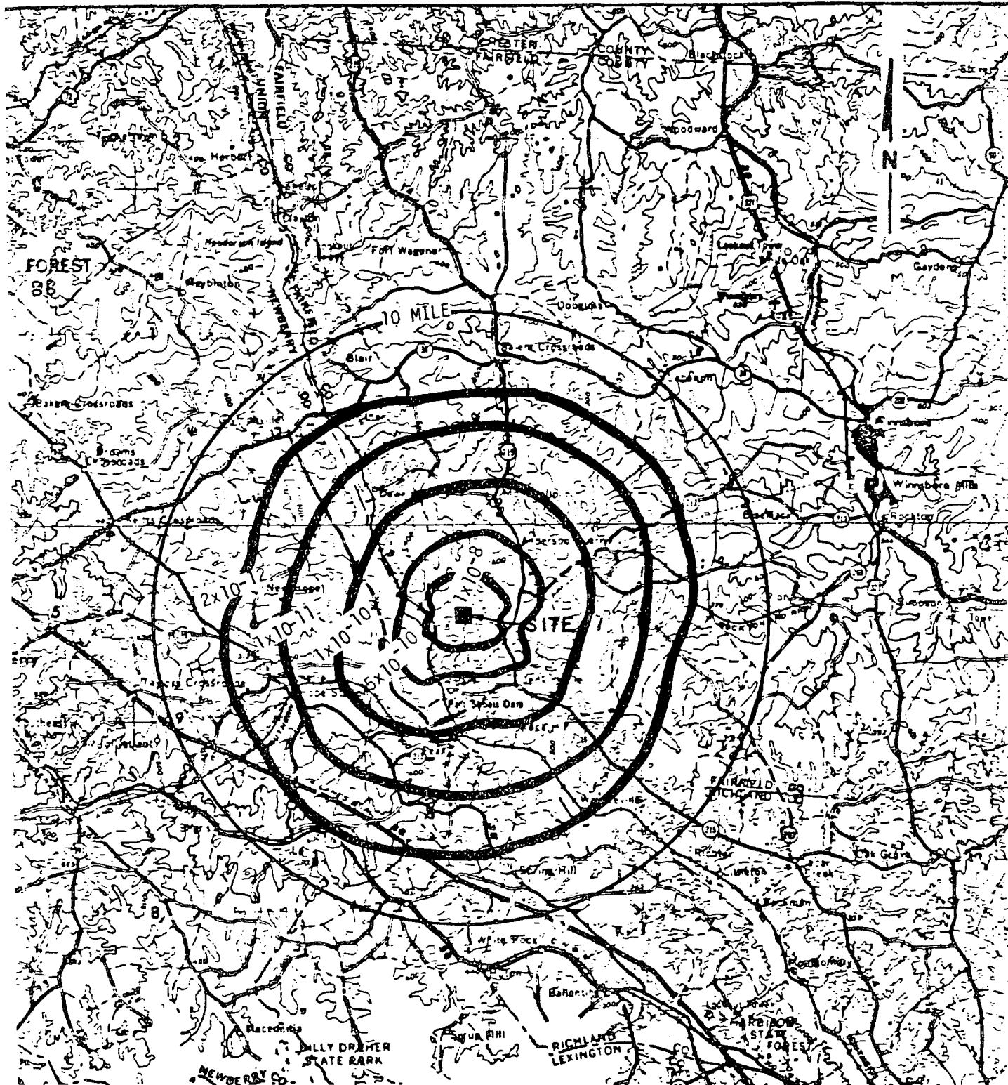
ISOPLETHS OF RISK OF ACUTE FATALITY PER REACTOR YEAR TO AN INDIVIDUAL
