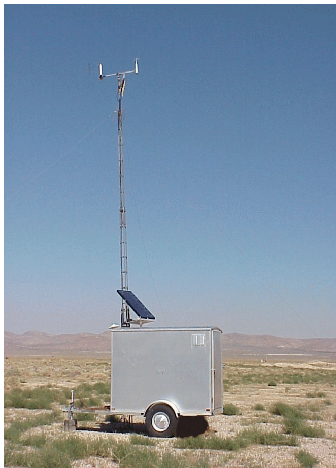
Figure 16-1. Example of a typical MEDA station with a 10-meter tower
