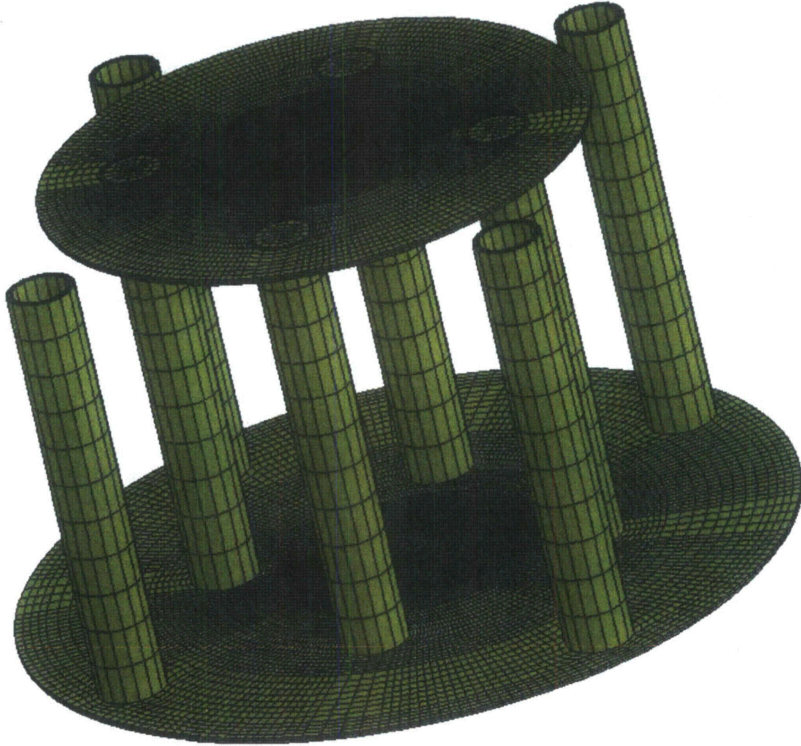
Figure 25: Ring Assembly Shoring; Meshed
