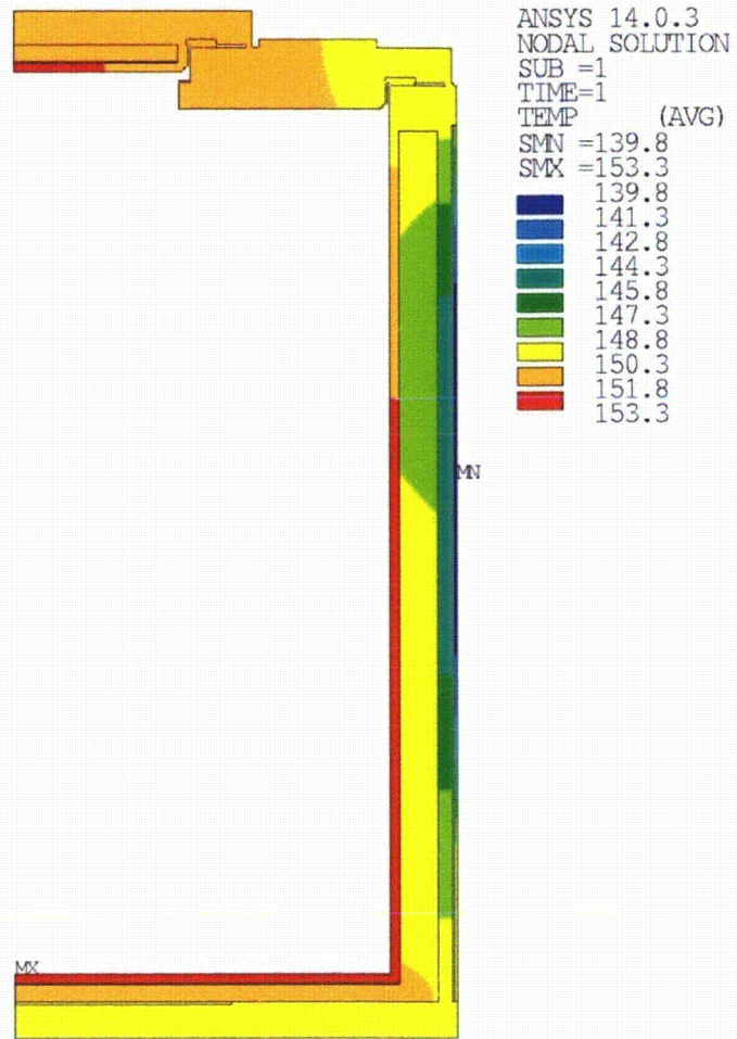
Figure 2-12 – Hot Environment Temperature Distribution (Reproduced from Figure 3-5)
