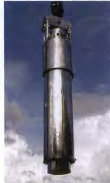
NAC LWT spent fuel transport package is moved by crane. (Courtesy: NAC International)
