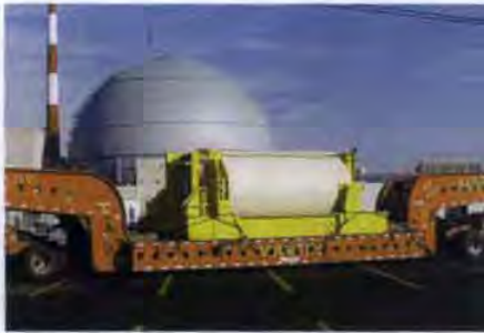
Transportable spent fuel storage cask moves to storage pad.
