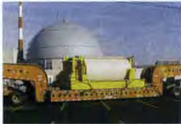
Transportable spent fuel storage cask moves to storage pad. (Courtesy: Holtec International)
