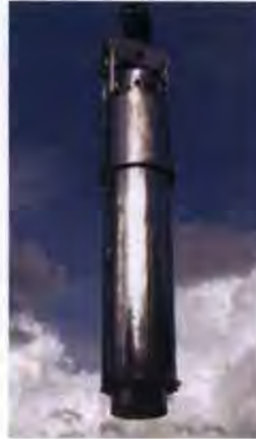
NAC LWT spent fuel transport package being moved by crane.
