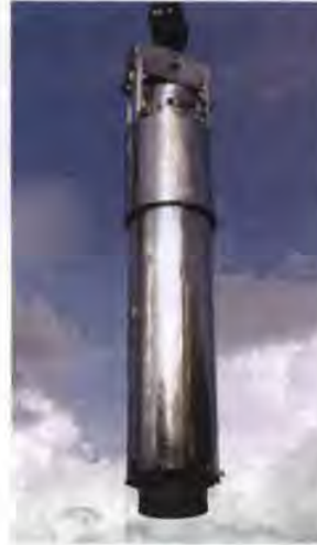
NAC LWT spent fuel transport package is moved by crane. (Courtesy: NAC International)
