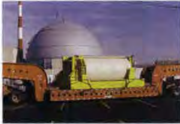
Transportable spent fuel storage cask moves to storage pad. (Courtesy: Holtec International)
