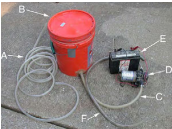
Figure C-5. Burrow pump employed for extraction of burrow co-inhabitants. A - intake hose, B - filtering bucket, C - water removal hose, D - 12 volt water pump, E - 12 volt battery, F - discharge hose.
