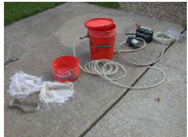
Figure C-6. Burrow pump parts. From bottom left to upper right; elastic band for securing filtering material, 2 filter cloths, internal filtering bucket, 5 gallon bucket with gasket lid, water pump, 12 volt battery, and optional size hoses.
