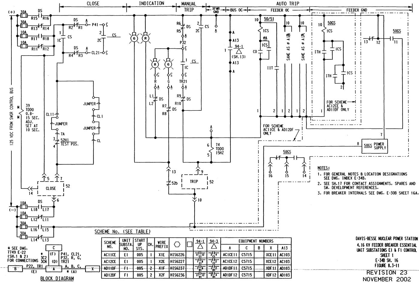
4.16 KV FEEDER BREAKER ESSENTIAL UNIT SUBSTATIONS EI & FI CONTROL
