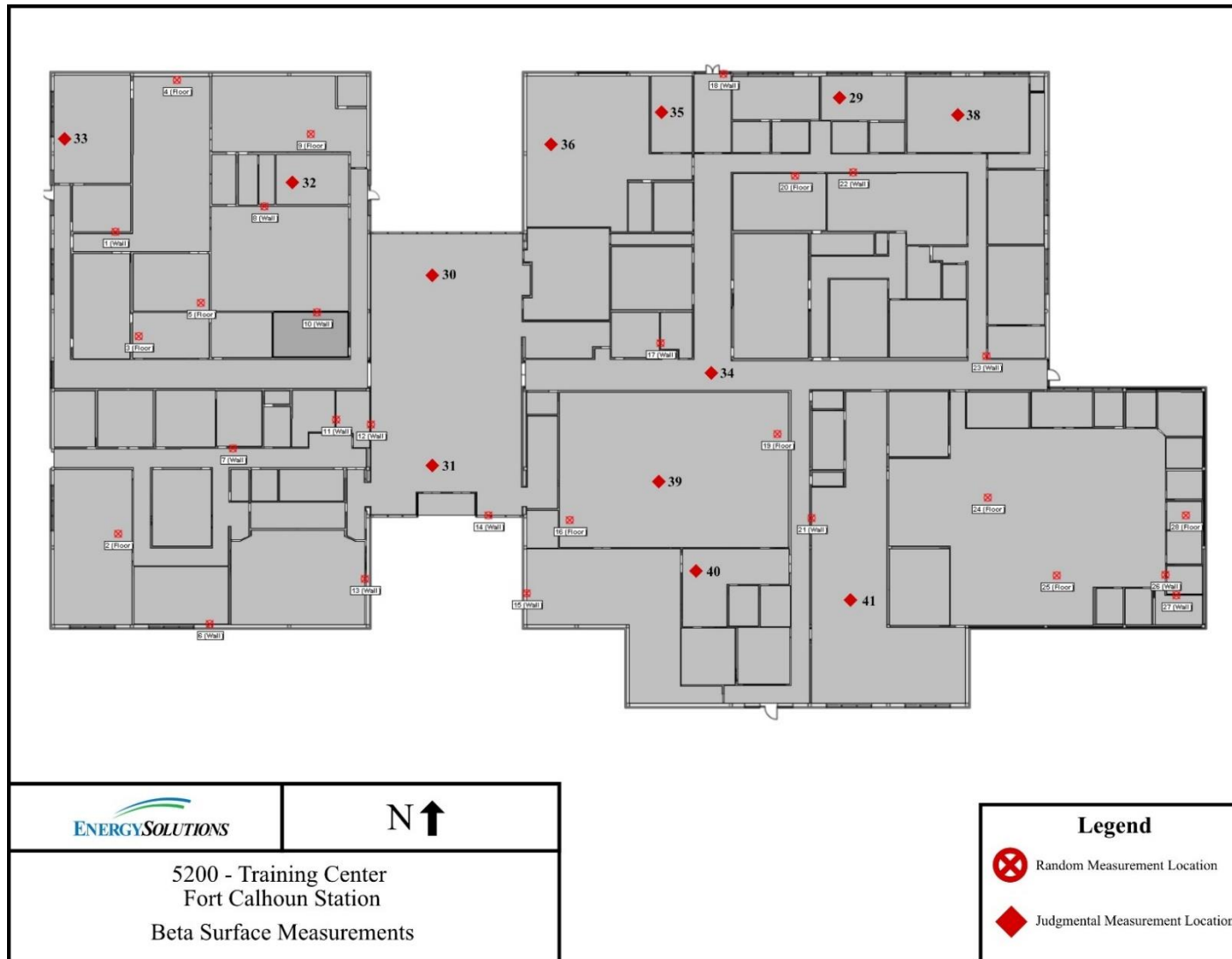
Figure 2-64 Training Center Surface Measurement Locations
