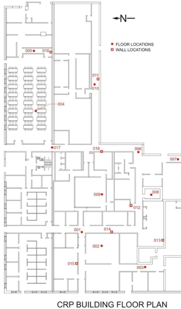
Figure 2-57 Chemistry and Radiation Protection Building Surface Measurement Locations
