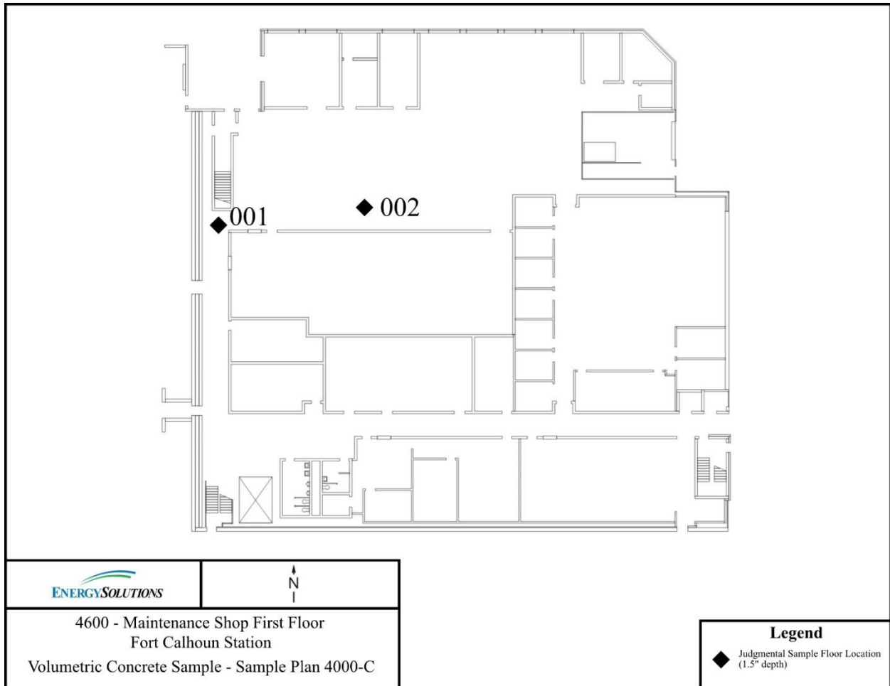
Figure 2-23 Volumetric Concrete Sample Location in Maintenance Shop
