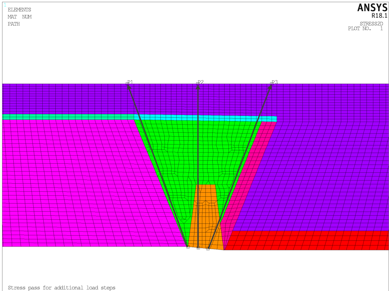
Figure 3: Path Locations for Through wall Stress Extractions for As-Built “Minimum” WOL Weld Residual Stress Analysis
