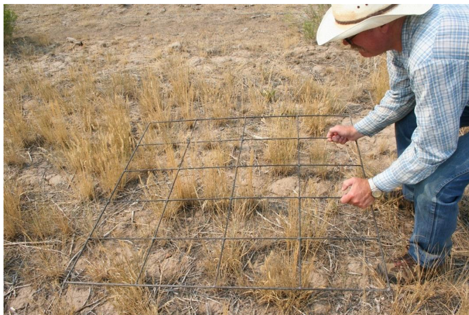
Figure 2. A density frame is used to measure plant density in a rangeland seeding.
