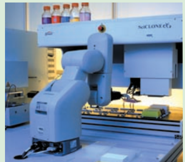
NREL scientists use a robotics deck such as this to quickly culture genetic variants of fungal genes for producing enzymes and screen them to identify the variants with the most promising characteristics.
