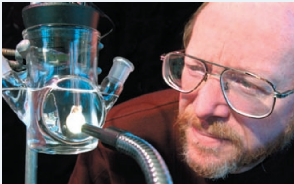
NREL scientist John Turner demonstrates the ability of a PEC cell to produce hydrogen from water using energy from a light source.
