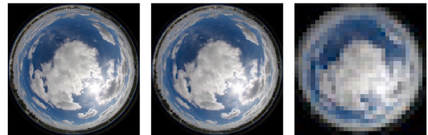
Fig. 11. Sky image at different pixel resolutions: 512 \times 512 , 128 \times 128 , 32 \times 32 . Source: SIRTA [129].
