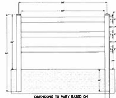
3 RAIL VINYL FENCE DETAIL NTS
