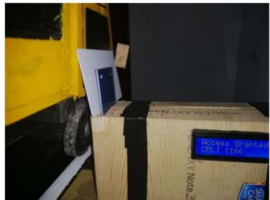
Figure 10-- IOT Device model- RFID UID reading process to grant the sand truck using LCD display 2 project has been addressed the Human Computer Interaction issues because of the most of time this mobile application will be used and accessed by the non-computer literate people. Less complexity and high user friendliness are provided to access the system without having unnecessary details.
