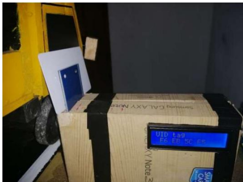
Figure 2-- IOT Device model- RFID UID reading process using LCD display
