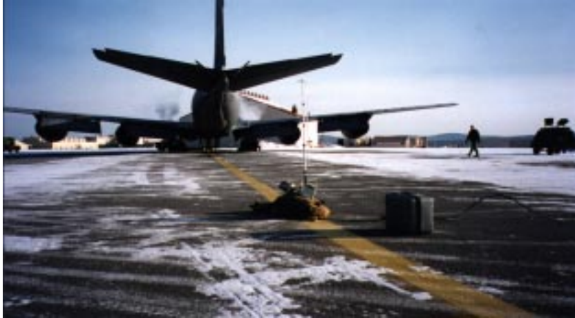
Measuring JP-8 aerosols and vapors in KC-135 exhaust at Eielson AFB, Fairbanks, Alaska, March 1997.
