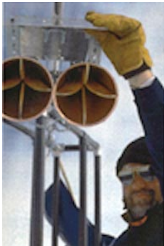
Two antenna horns of a radar instrument used to monitor the backscatter properties of snow and ice at the equilibrium line altitude.
