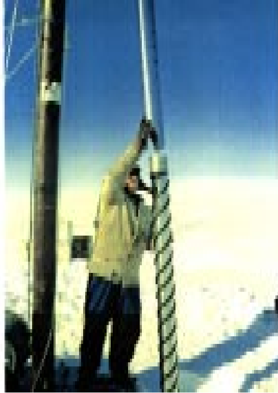
Drilling shallow cores to establish the historical accumulation and elevation of the ice sheet over the past few hundred years.
