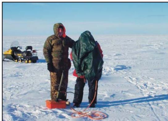
Data collection using ground-penetrating radar. The plastic bag is to exclude the bright ambient light and allow the operator to see the readout.
