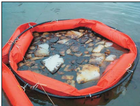
Dispersant experiment in cold water and broken ice at Ohmsett.
