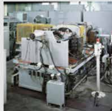
Test rig for bearings used in work rolls of rolling mills
