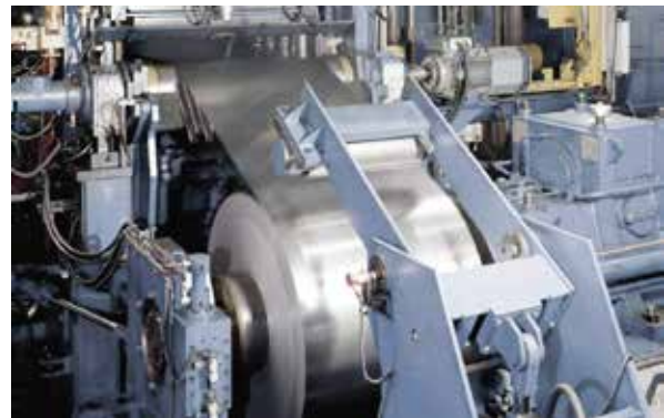
↑ Cold Rolling Mill
