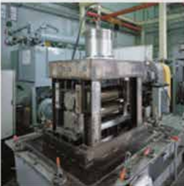
Test rig for bearings used in guide rolls of continuous casting machines
