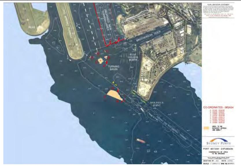
Figure 2.13. High spots in bottom profile requiring maintenance dredging as part of the port expansion proposal. Source: Sydney Ports Corporation.
